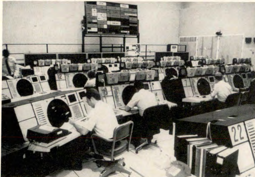
The Alaskan Region Operations Control Center consolidates radar data and provides nearly instantaneous transfer of information to the North American Aerospace Defense Command.
